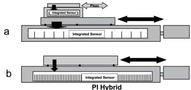
Different types of combined motorized and piezo positioning systems:
